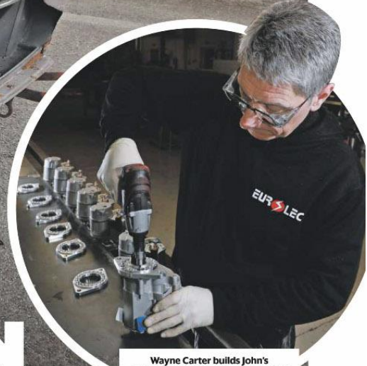
Wayne Carter builds John's adjustable starter motor. The swivel mount was originally designed for race cars but also provides maximum adaptability when swapping engines.
