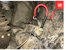
cable provided to the M4 bolt on the new RAC680 Alternator ensuring not to over tighten.
