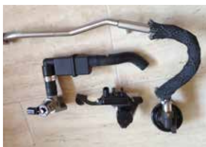
The ERG Valve, the Fuel sensor and the Idle control valve, all superfluous to requirements.
